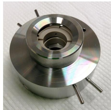
6 sets of ver 5 of the mini-bioreactor with 5 ml scaffold was manufactured purely in AISI316 steel. One of several advantages of the latest design is that the scaffolding envelope can easily be altered in height from almost zero to 6 mm. The flow of media is laminar through and perpendicular to the scaffold.
