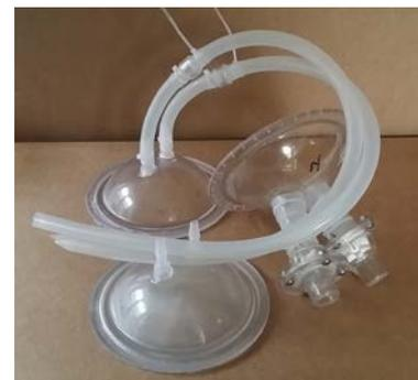
The dome is sealed with a thin silicone membrane dividing the sterile wetted internal volume from external non-sterile environment. One or more hoses connect to inlet, outlet, valves, pinch valves for control of liquid volume and direction. This SUP eliminate the typical need for peristaltic pumps.
