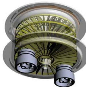
Cells arranged in scaffold being electrospun organic fibres into discs assembled inside 2 envelopes in SUB.
