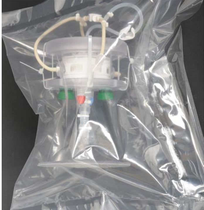
Finished 50 ml scaffold volume HESUB all pre-assembled and packed in dual film bags before precision E-beam irradiation. Sensors for pH, DO, Glucose, Lactate installed in the media reservoir. Ready for use.
