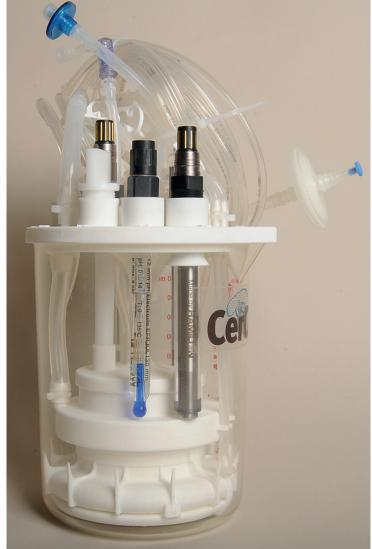
Perfusion is a method for continuous cultivation, where cells are harboured inside a 3D matrix / scaffolding and a steady flow of nutrients are fed to the cells, giving a continues harvest for an extended period.
