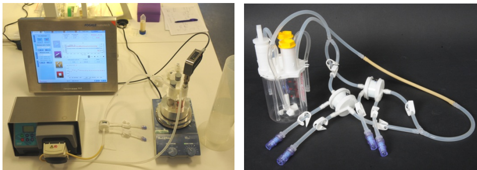
One CellVessel 21-0250 STR connected in series with one or more CellCompact Macro Perfusion SUBs and a peristaltic pump able to re-circulate 100 ml/min media.
