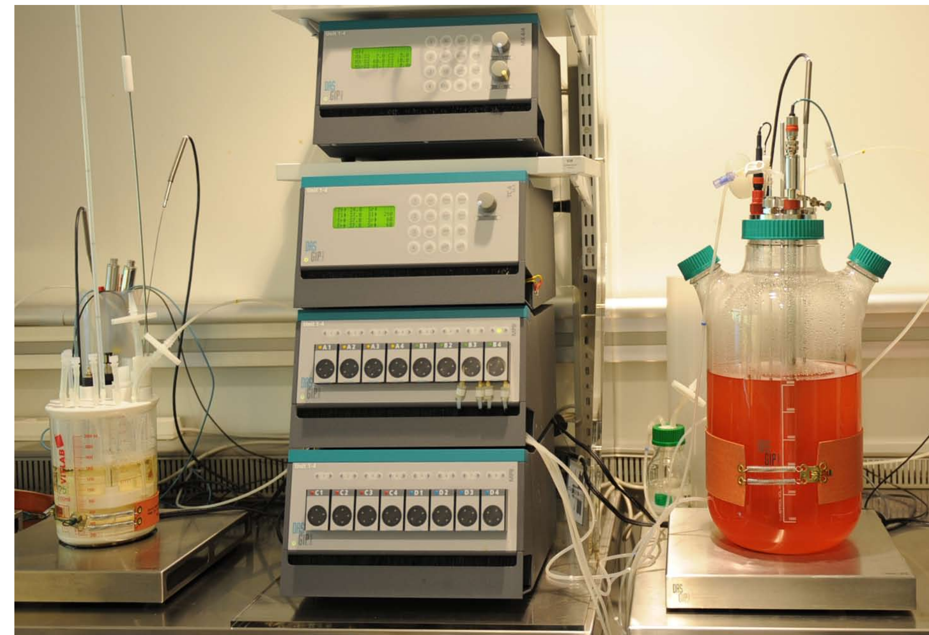
Photo 1 - Lab testing at Bioneer in Denmark (November 2011) of the CellTank p/n 22-0150 perfusion SUB on DasGip MP8 Process-Control-System (PCS) with identical suspension CHO cell line compared against an autoclaved 8 litre glass STR. Both STR and SUB had identical 1.5 \times 10^{10} cells. The SUB with 150 ml matrix volume/1 litre reservoir volume operates for weeks in perfusion setup. The traditional STR with CHO cells in suspension and 6 litre working volume was cultivated for 6 days before termination as to extensive lactate levels.
