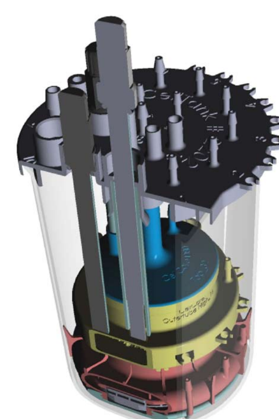
Sketch 1 - 3D cut through the CellTank p/n 22-0150 illustrating at left the 120 mm pH SUS and at right the re-usable VisiForm PG13.5x160 dO 2 sensor fitted to the non-invasive well with the permeable membrane in the front. Slightly visible behind pH is the 120 mm SUS bio mass sensor.
