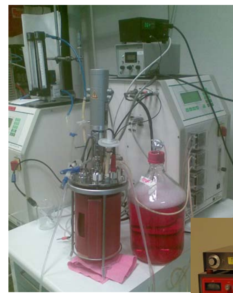
Photo 2 - CellTank p/n 22-0150 SUB tested at Bioneer on DasGip MP8 PCS with suspension CHO producing IgG compared against a 600 ml working volume conventional glass/steel STR. The SUB reached cell density of 0.8 \times 10^8 cells/ml, for continues perfusion of 2 litre exchange/day. Graph 1 and 5 at left. Application Notes on www.cerccell.com
