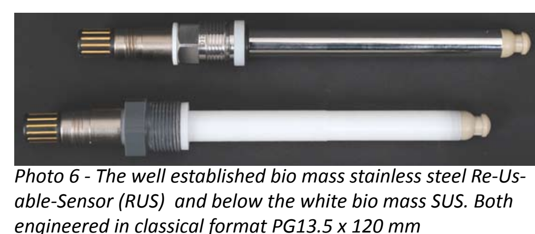
Photo 6 - The well established bio mass stainless steel Re-Use-Sensor (RUS) and below the white bio mass SUS. Both engineered in classical format PG13.5 x 120 mm
